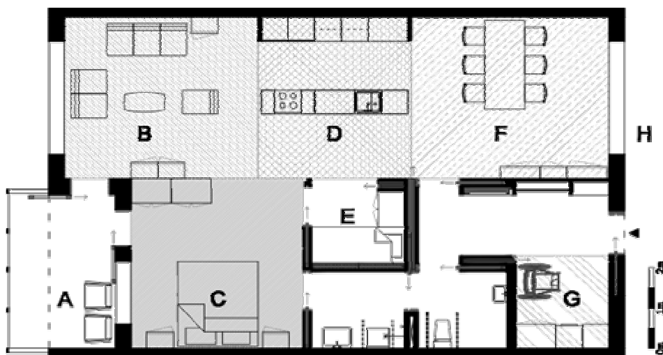
Figure 1 Basic design for Aging-in-Place. A: Balcony: not used at first, semi-public later; B: Living area at first, semi-public dining and semi-private bedroom area later; C: Private: bedroom, living area later; D: Open kitchen: Semi-private to semi-public; E: Semi-public multiple use area; F: Semi-public: dining and living area; G: Storage space (multifunctional); H: Outdoor public space.
