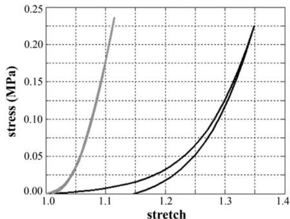
Fig. 2. Hysteresis for young (black line) and aged (grey line) viscoelastic tissues for a tensile loading-unloading cycle. The dissipated energy is represented by the area in between loading and unloading curve.
