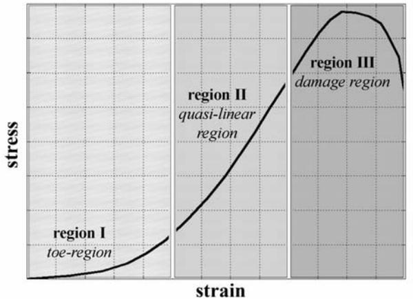
Fig. 1. Typical stress-strain behavior of a connective tissue rich in collagen fibers, up to failure.
