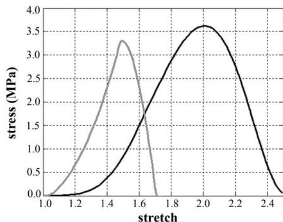
Fig. 3. Monotonic tensile behavior for young (black line) and aged (grey line) tissues up to the total failure. The dissipated energy is represented by the area under the stress-strain curve.
