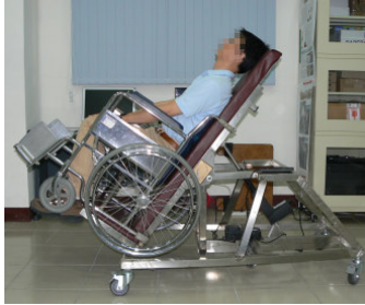
Fig. 2. The prototype electrical controlled tilt-in space pressure-relieving system with regular wheelchair user.
