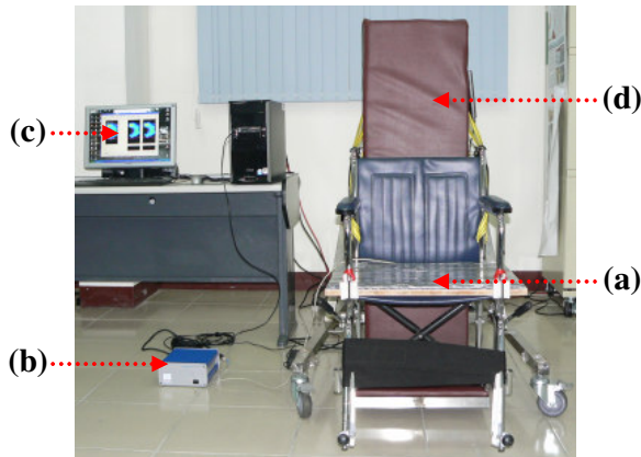
Fig. 4. The integration of experiment system. The wheelchair, the prototype electrical controlled tilt-in space pressure-relieving system, and RS Scan F-Scan pressure measuring system: (a) F-scan USB
