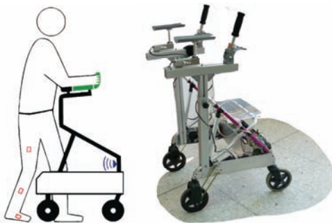
Fig. 8. Subsystems and a picture of the SIMBIOSIS walker.
