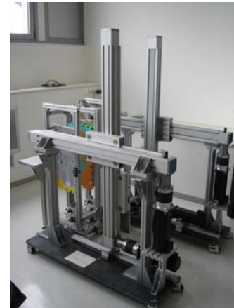
Figure 8: Realization of overall structure of NEUROBike
