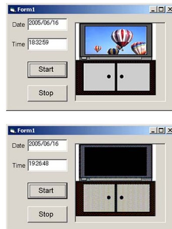
Fig. 2. Upper and lower windows indicate on the computer at the family's end. Upper window: TV-on; Lower window: TV-off.
