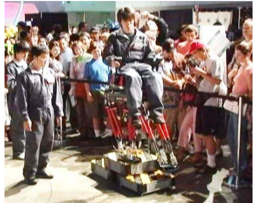
(a) The robot goes up and down stairs with the rise of 150 mm and the pedal tread of 300 mm continuously.
