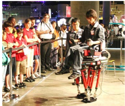
(b) The passenger navigates the robot by using the control stick mounted on the passenger seat.
