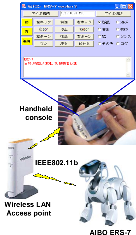
Fig.8 Remote control system developed for use by the therapist
