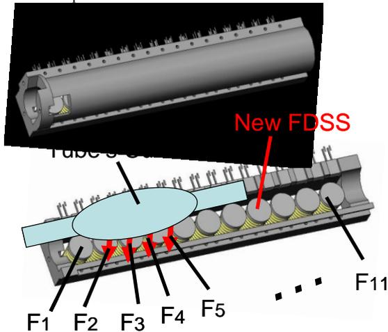
Fig. 9 Details of the redesigned trachea of the WKA-1R in order to embed the improved FDSS.
