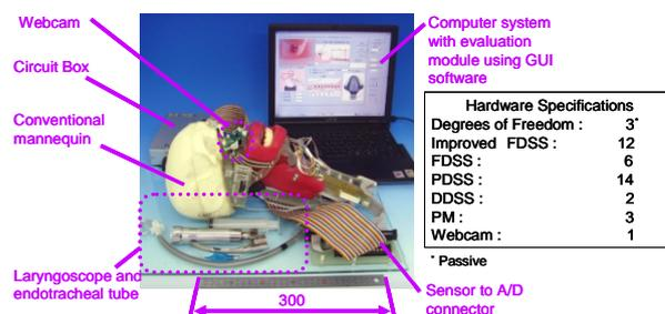
Fig. 1. System overview of the newest Waseda Kyotokagaku Airway No.1R (WKA-1R). This new version has improved the designing of the Force Detection Sensor System to measure better the applied forces while performing the task.
