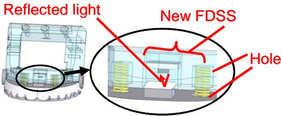
Fig. 8 Details of the redesigned incisor teeth of the WKA-1R in order to embed the improved FDSS.
