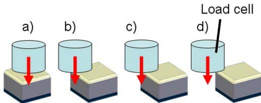
Fig. 4 Experimental conditions to determine the curve characteristics of the proposed FDSS designed for the WKA-1.
