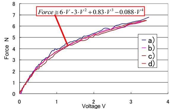
Fig. 7 Characteristic curves obtained by the improved FDSS designed for the WKA-1R (a, b, c, and d are the different considered cases shown in Fig. 4).
