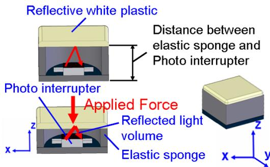
Fig. 3 Details of the Force Detection Sensor System designed for the WKA-1 [19].
