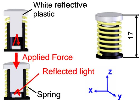
Fig. 6 Working principle of improved FDSS designed for the WKA-1R.
