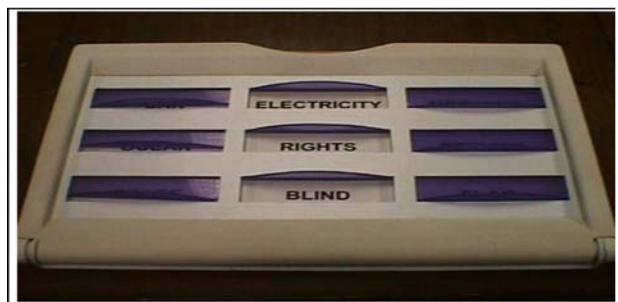
Fig. 5. The Mock-up features an adjustable tilt device with hinges visible at the front and top to bottom sliding windows. The tilting mechanism is flat and not contoured to a persons lap. The top to bottom shades were easy for players to learn, required minimal effort, and were found to be the optimal covering system.
