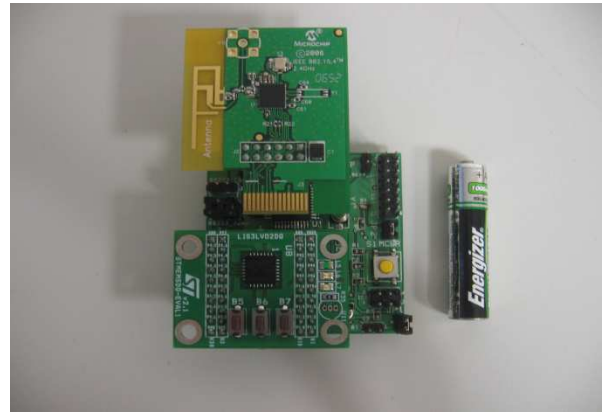
Fig. 1. The wearable sensor prototype.
