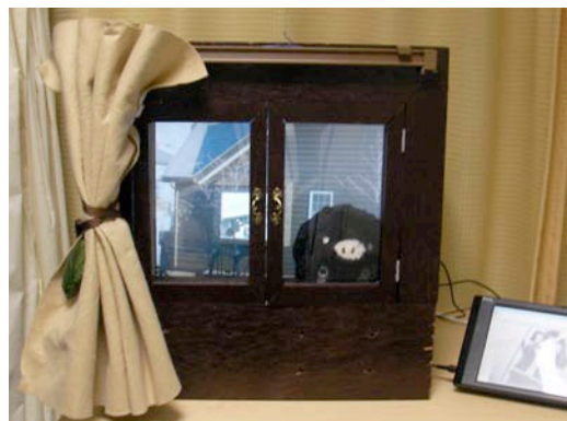
Fig. 2. External appearance of the implemented prototype system. A touch-screen LCD is installed inside a wooden window frame and displaying the view of the “next-door” house. Video image transmitted from the remote site is displayed inside the large window of the house.
