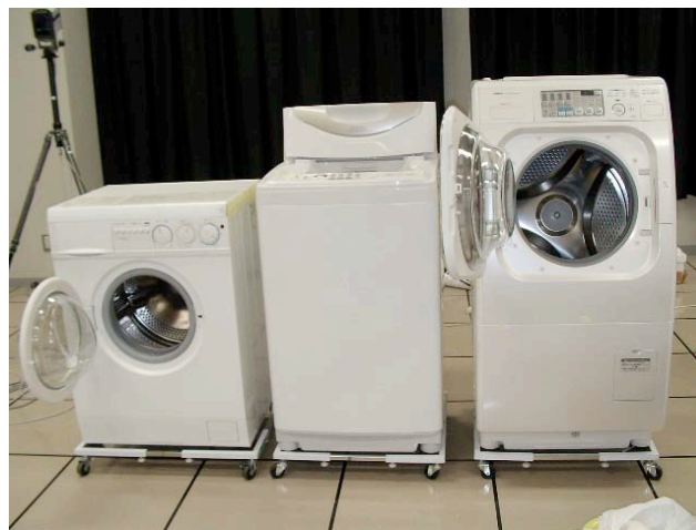
Fig.1. Washers and a New Washer-Dryer; European (EU) type AWD-500, Vertical Drum type ASW-800 and Slanted Drum type washer-dryer AQ-1(Left to Right).
