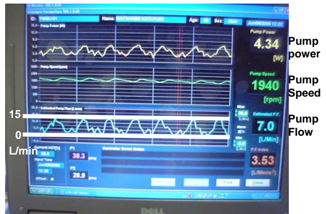
Fig. 9. Typical monitor screen of hemodynamic waveforms during EVAHEART pumping (case 1)
