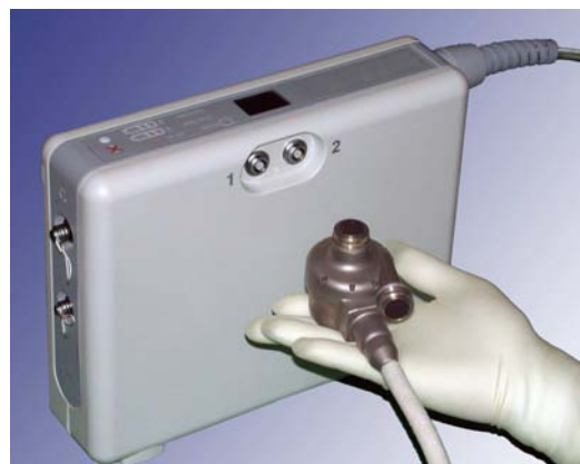
Fig. 1. EVAHEART system for final prototype (clinical) model
