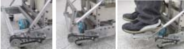
Fig. 3 The rotatable electrically operated swing foot pedal instalment
