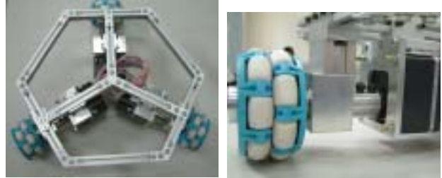
Fig. 1 The mechanical structure of the omni-directional wheelchair
