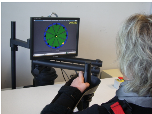
Figure 2. A patient during the robot-mediated therapy (standard robotic therapy rehabilitative scenario)
