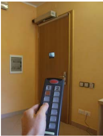
Figure 9: A test with a simplified remote control used to control the domotic system
