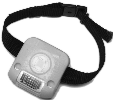
Figure 1. RTLS wristband with compact tag used in this study. It is both small and wireless, making it useful in this domain
