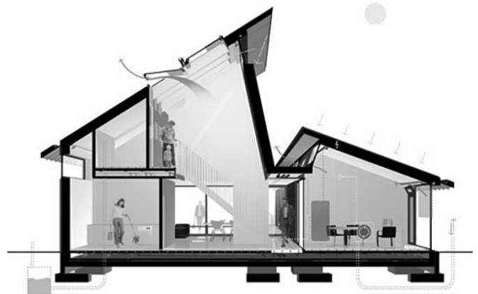
Figure 1. Cross section of the HoTT project showing day light penetration, ventilation principle and the aorta regarding services in the centre of the house facilitating Slimbouwen process
