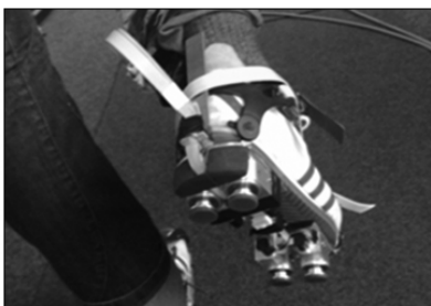
Figure 1. TUKE design of the rehabilitation shoe (left); 1 Change of gait speed over the first training period (right)
