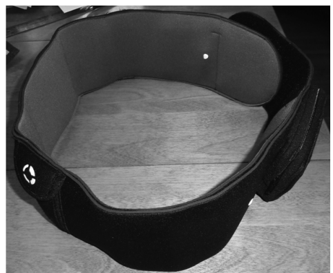
Figure 1: Tactile navigation belt consisting of a controller and 4 vibrotactile actuators
