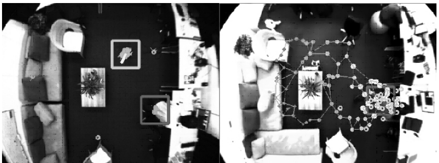
Figure 1. Ceiling-camera view of an apartment; Left: A person and a robot are localized; The spots are particles for the robot and the user; Right: The units and the links of the built cognitive map
