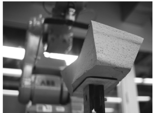
Figure 1. Mass customized robotic fabrication of wire-cut ruled-geometry clay elements for complex ceramic structures
