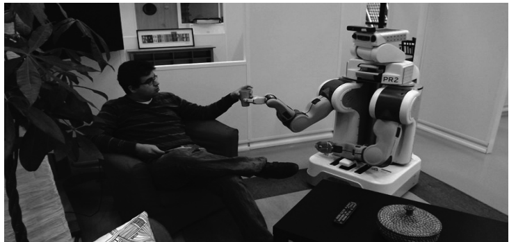
Figure 2. The exchange is comfortable for the human user who sees the robot and can take the object safely; The robot watches the human user and monitors the exchange process
