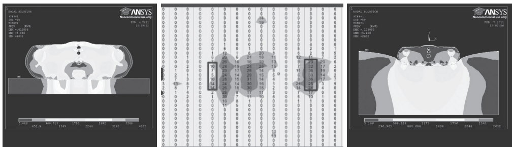
Figure 1. Computational result showing an upper shoulder model on a YM 25kPa mattress (left); actual measurement results with a 63kg male (center) and a softer YM 3.81kPa mattress model (right)
