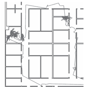
Figure 3. Facility floor plan revealing tracking data from Ubiwatch; Area represents approximately 30m x 21m
