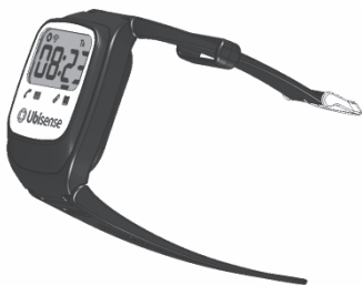
Figure 1. Ubiwatch ordinarily displays time and day of the week; A programmable display shows four-character strings such as PILL or APPT; Pressing the display face requests help
