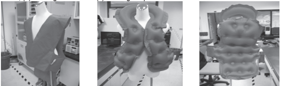
Figure 2. Experimental observations on the inflating process of the wearable airbag
