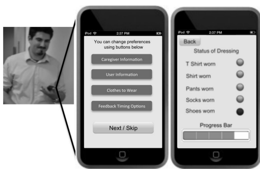
Figure 2. Caregiver system's interface. Examples of 2 iPod screens with system settings menu (bottom left) and status of dressing progress (bottom right). © Mahoney & Burlleson
