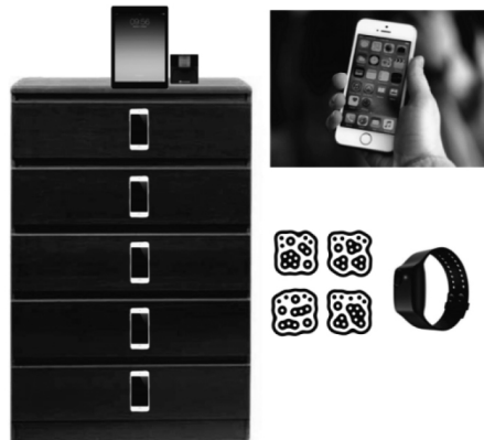
Figure 1. DRESS alpha system, smart dresser system components: dresser, iPad, motion sensor, iPods, caregiver mobile device, fiducial barcodes, and wrist sensor
