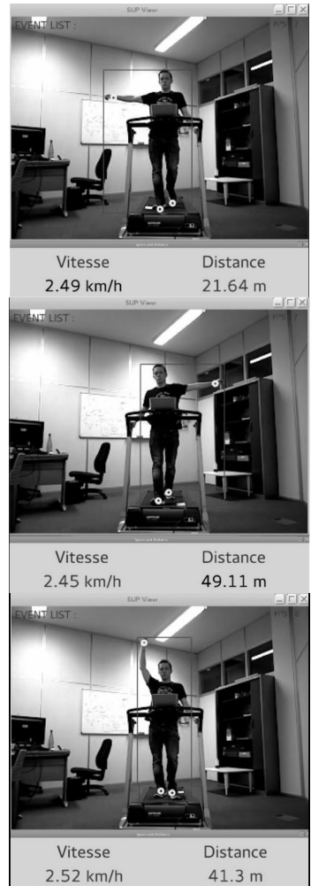
Figure 1: Gesture recognition and walking speed computation for serious game interactions; The gestures are: turning right (upper), turning left (middle) and action (lower); dots show the positions of arm and feet
