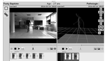
Figure 2: Screenshot of the interface for a rehabilitation application; Top: patient general information; Left: camera image; Right: 3D side view of the cloud of points of the person; Bottom (thumbnails): sequences detected in the video
