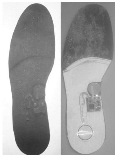
Figure 1. The smart insole used in the living lab experiment; LEFT: First laboratory tests showed good reliability measures and also a good acceptability by the users 2 ; RIGHT: the printed circuit board includes the following elements: a low-power 3-axis acceleration sensor, a microprocessor unit and a transceiver, a flash memory card and a nano-powered time keeper to activate scheduled data-logging modes.
