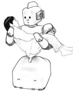
Figure 1. The lifting robot Ri-Man 4 , carrying a mannequin (drawing by the author)
