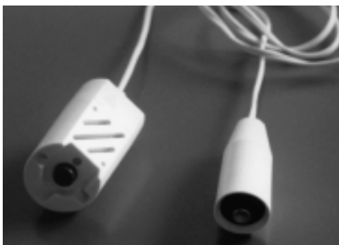
Figure 2: Bedside call-button device provided for in-patients in a geriatric rehabilitation hospital
