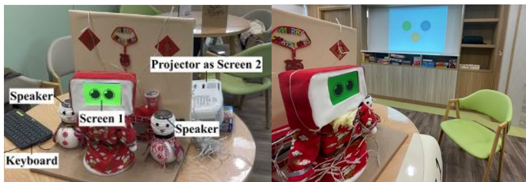
Figure 1. Social robot with full setup (Left), Project screen sample output with the setup (Right)
