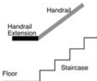
Figure 4. Handrail extension. It continues from a staircase handrail and are level with the floor at the top and bottom of a staircase.
