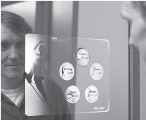
Figure 2. MyHeart (Royal Philips Electronics) allows for real-time monitoring of a persons body signals, such as activity level, which could be used as input parameter for HVAC-control. MyHeart can be integrated into wearable garment, while a mirror contains a display for user interaction. Source: http://www.research.philips.com/newscenter/pictures/downloads/health_pershealth_06_h.jpg
