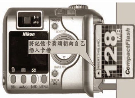
Figure 2. A snapshot of the animated visuals dynamically exhibiting the push-in and pull-out of a memory card; Chinese text reads: 'Hold the memory card with the arrow facing towards you and insert the card in the direction of the arrow'
