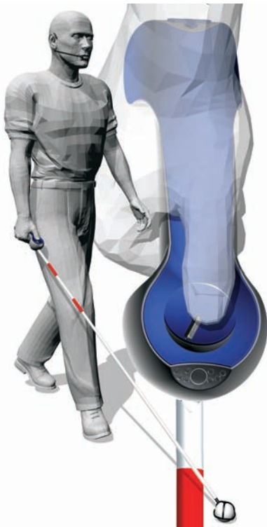
User interface of guide cane. The arrow pointing in the correct and safe walking direction is felt by the thumb
