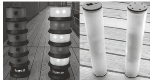
Figure 2. Light & Sound cylinders consisting of a base unit and five Light & Sound units (LSUs, left), and Rolling Pins (RPs, right)
