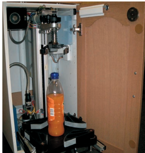
Figure 1. MAGIC-HAND: Left: Computer design drawing of the bottle and jar opening mechanism comprising a base unit, a vertical linear actuator and a top unscrewing unit; Right: The assembled opening mechanism is secured on a sliding tray inside a standard 400 mm wide kitchen unit; The electromagnetic lock is shown at the top-right corner of the door
