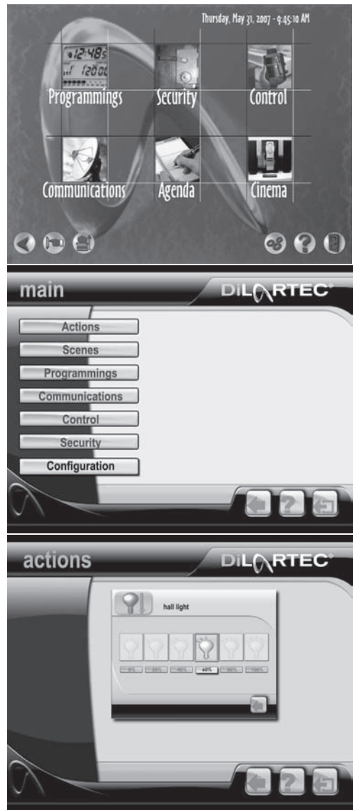
Tactile screen interface of LARTEC's Domotic System before (upper picture) as tested in the experiment and new non-tactile interfaces after applying the results of emotional engineering (middle picture: main menu; and lower picture: a sub-menu)
