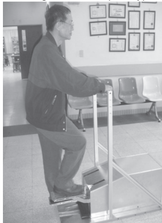
Figure 2 A finished prototype of the step machine was using by the simulation of elderly
