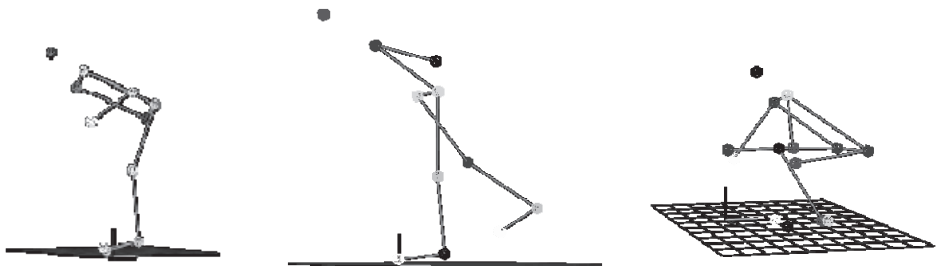
Figure 1 Motion captured posture of picking laundry from drum bottom. Left to right; Slant drum (New product), Vertical drum (conventional type which popular in Japan) and horizontal drum (European type)
