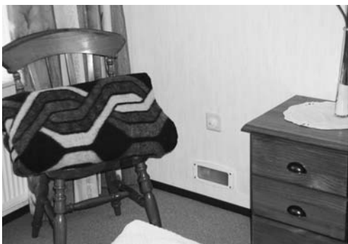
Figure 4. Passive infrared sensor with night light below
