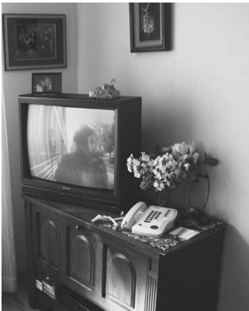
Figure 2. Access control: watching TV, speak via the alarm phone and push button on the phone to open the door remotely
