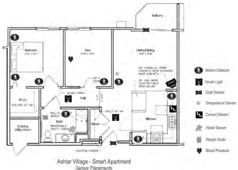
Figure 1. Schema of sensor placement in a typical apartment in the study site
