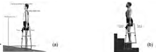
Figure 1. Phase a Concept Design: The topography adaptable walker, (a) on slope; (b) on stairs
