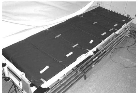
Figure 1: Hospital bed with pressure sensor array (mattress is placed on top)
