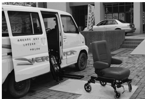
Figure 2. The prototype of the electric auxiliary seat
