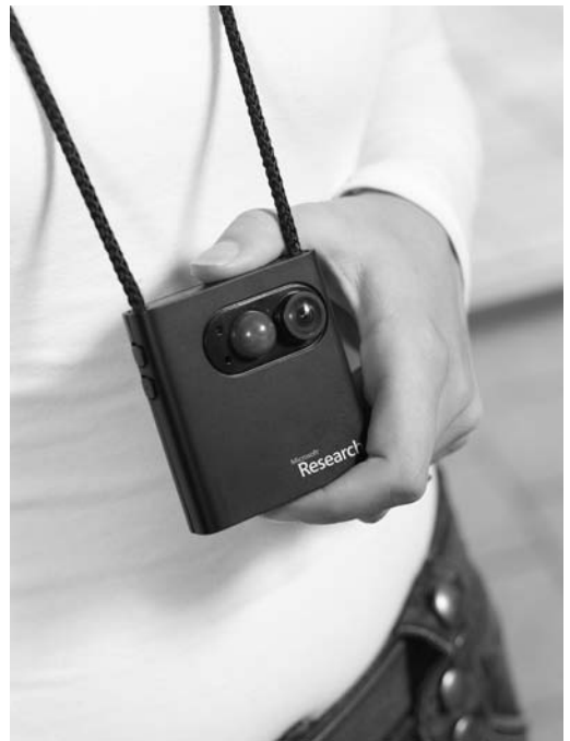
Figure 4. SenseCam: A wearable camera that can automatically take pictures to supplement memory
