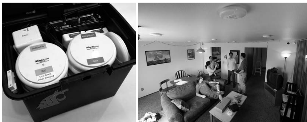
Figure 1. CASAS 'smart home in a box' kit (left) and smart home installation site (right)
