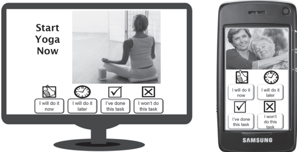
Figure 2. CASAS prompts can be sent to a touch-screen device (left) or to a mobile device (right). The text and audio content can be automatically generated, and the user may choose to respond to the prompt or ignore it
